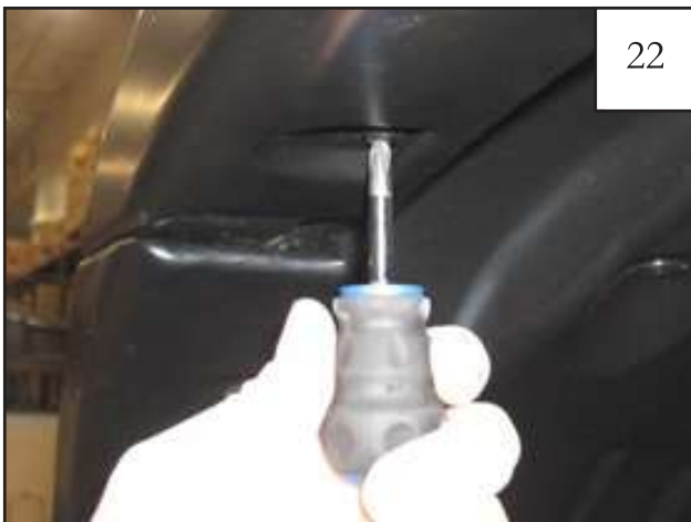
Install a supplied Phillips Truss Screw (SW1-0050) through hole in flare and into Clip installed in Step 19
